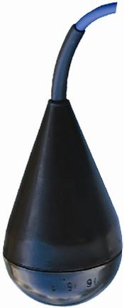
The MS1 EX float switch can be used in a certified, intrinsically safe circuit electrical system for the control and regulation of liquid levels in Zones 0, 1 and 2 Ex- areas. It can also be used in the presence of gas groups IIA, IIB and IIC, where there is a risk of explosion when these are in contact with flammable materials and exposed to temperatures in the range T1 - T6.
