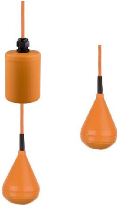
The M2 level regulator is a single-point regulator, specially designed for use in wastewater treatment plants and in pump stations which handle liquids polluted with solids. Thanks to its good chemical properties, it is resistant to a wide range of liquids.
